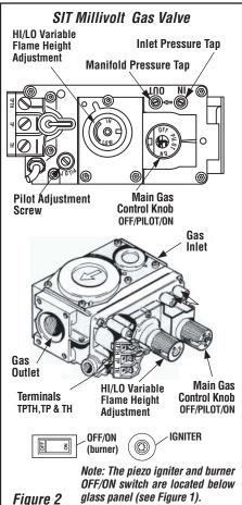
**Note:** To prevent excessive resistance in burner circuit (which can cause burner operation problems), only one burner control switch should be wired to valve. Therefore, if an optional control switch is installed, the standard Off/On switch and wires should be removed.
